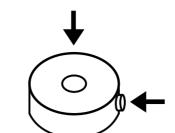
Two options for cable gland installation: at the top or at the side
